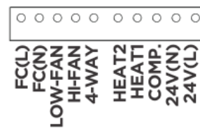
Terminal of PTAC Wall Thermostat (MODE B)
