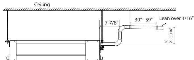
**NOTE:** When connecting multiple drainpipes, install the pipes as illustrated.
