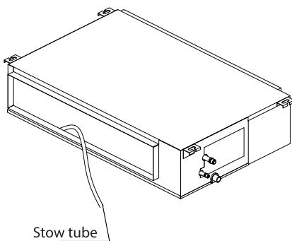
Fill the water pan with 2 quarts of water. Check that the drainpipe is unhindered.
